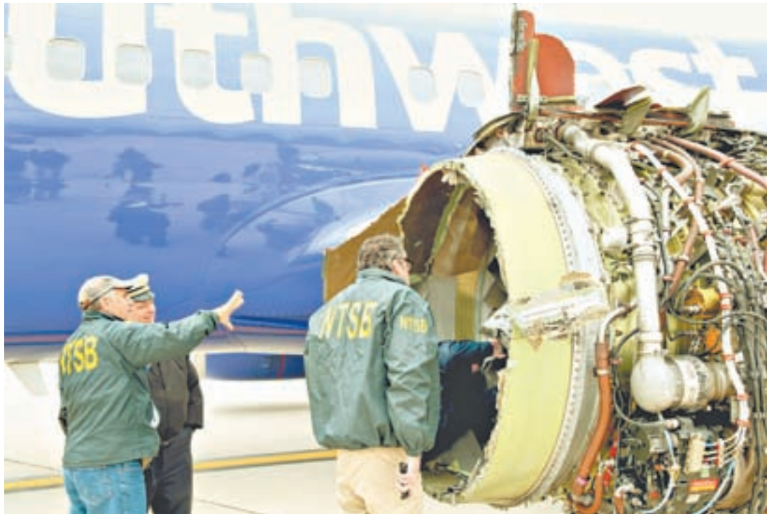
Investigators examine damage to the engine belonging to Southwest Airlines Flight 1380 that separated during flight on April 17, 2018 in Philadelphia, Pennsylvania. Investigators can't explain with certainty why the engine malfunctioned but are directing their attention to metal fatigue on fan blades. One woman died due to the incident. (Photo Keith Holloway/National Transportation Safety Board via Getty Images)
